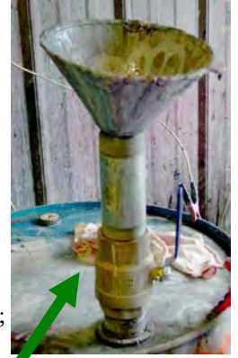
This funnel has a threaded discharge tube and a valve closure device.
